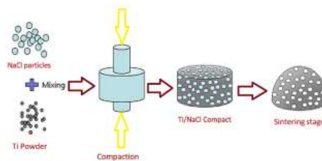
Figure 2: Synthesis of titanium foam.
