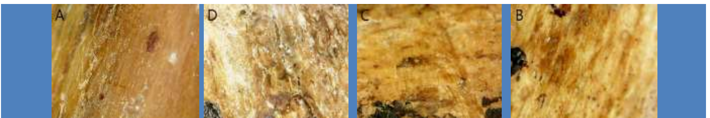
Fig (3) DM shows samples of nano paraloid 3% where (A) represents the standard sample ST and (B) the Strengthening sample NP and (C) a thermally aging Strengthening sample NPH (D) a chemically aging Strengthening sample NPK
