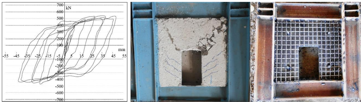
Fig. 1 . Hysteresis load-displacement curves and the damaged control specimens
