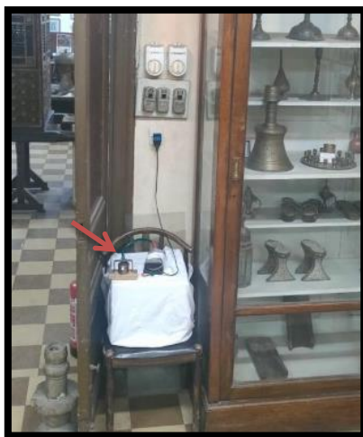
Fig .2 The figure illustrates the air suction pump utilized for the collection of dust samples at the study site.
