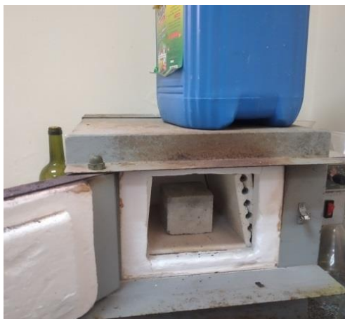
Fig. (7) Standard cube in electric furnace
