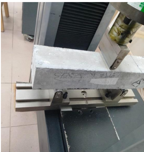
Fig. 5 Flexural strength test
