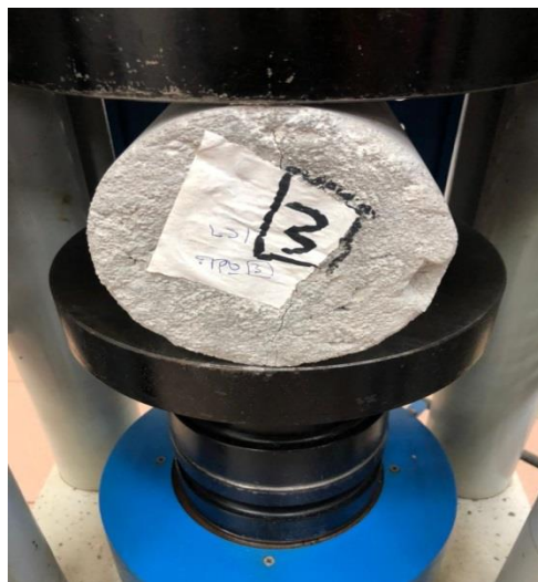
Fig. 6. Splitting tensile test
