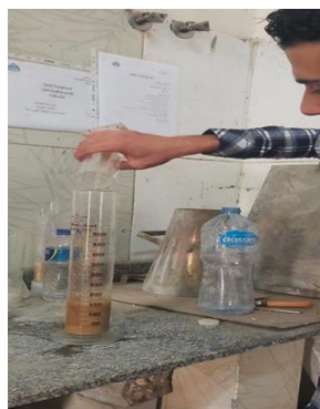
Fig. 2. determination of clay and other fine materials in fine aggregate by volume
