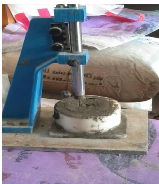
Fig. 1. Initial setting time test for Portland cement
